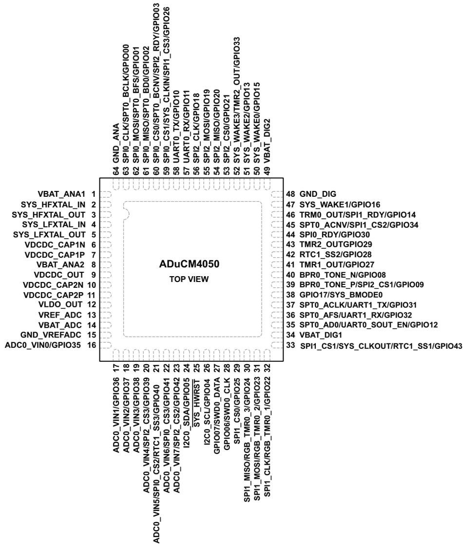
Figure 19. 64-Lead LFCSP Configuration
