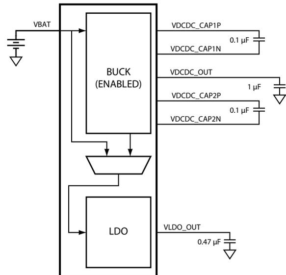
Note: For designs in which the optional buck is not used, the following pins must be left unconnected—`VDCDC_CAP1P`, `VDCDC_CAP1N`, `VDCDC_OUT`, `VDCDC_CAP2P`, and `VDCDC_CAP2N`.
