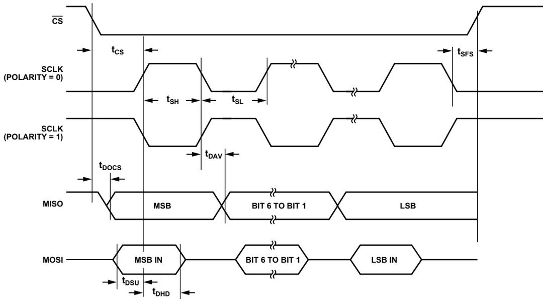
Figure 11. SPI Slave Mode Timing (Phase Mode = 0)
