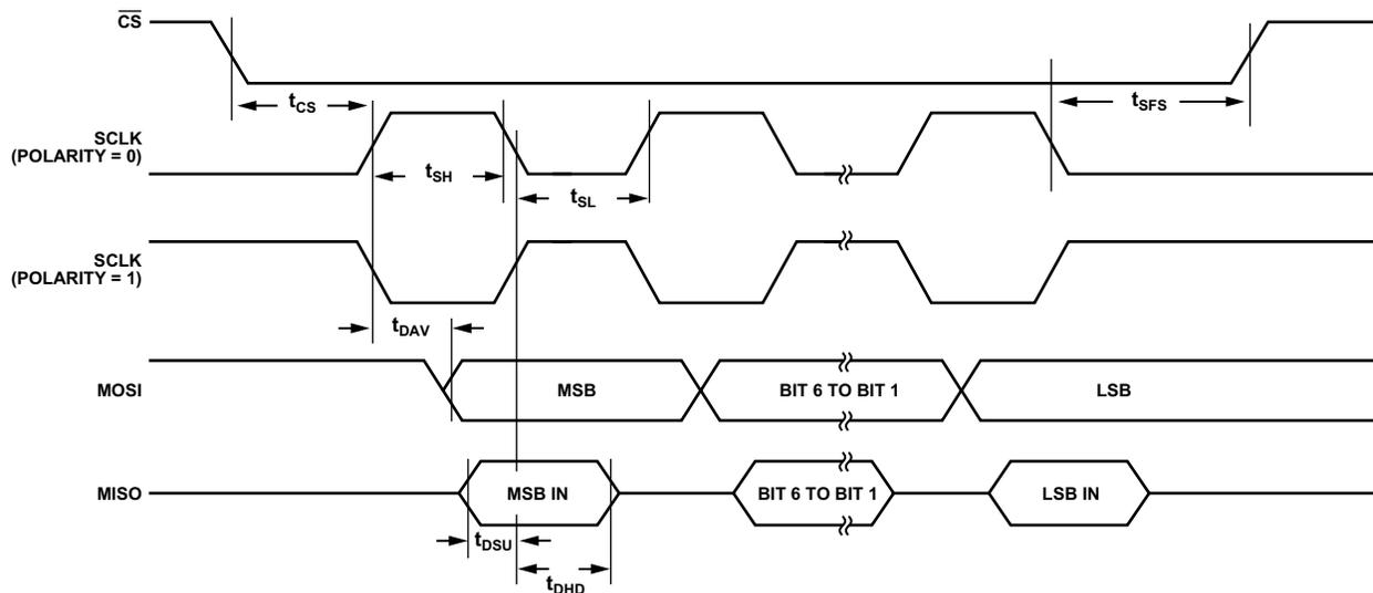
Figure 8. SPI Master Mode Timing (Phase Mode = 1)
