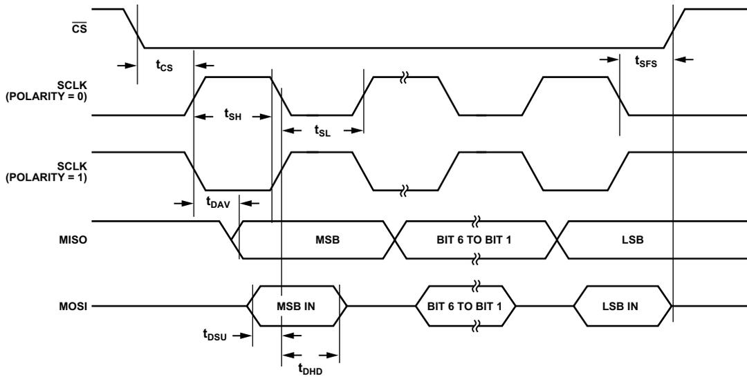
Figure 10. SPI Slave Mode Timing (Phase Mode = 1)
