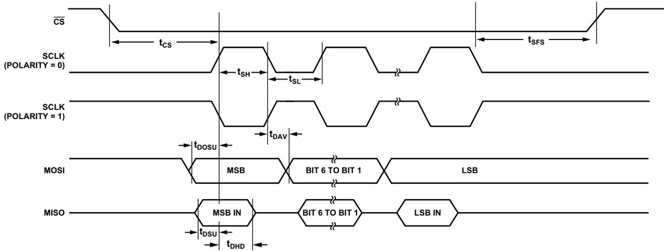
Figure 9. SPI Master Mode Timing (Phase Mode = 0)
