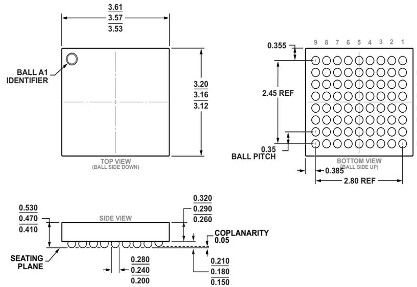
Figure 20. 72-Ball Wafer Level Chip Scale Package (WL CSP)
