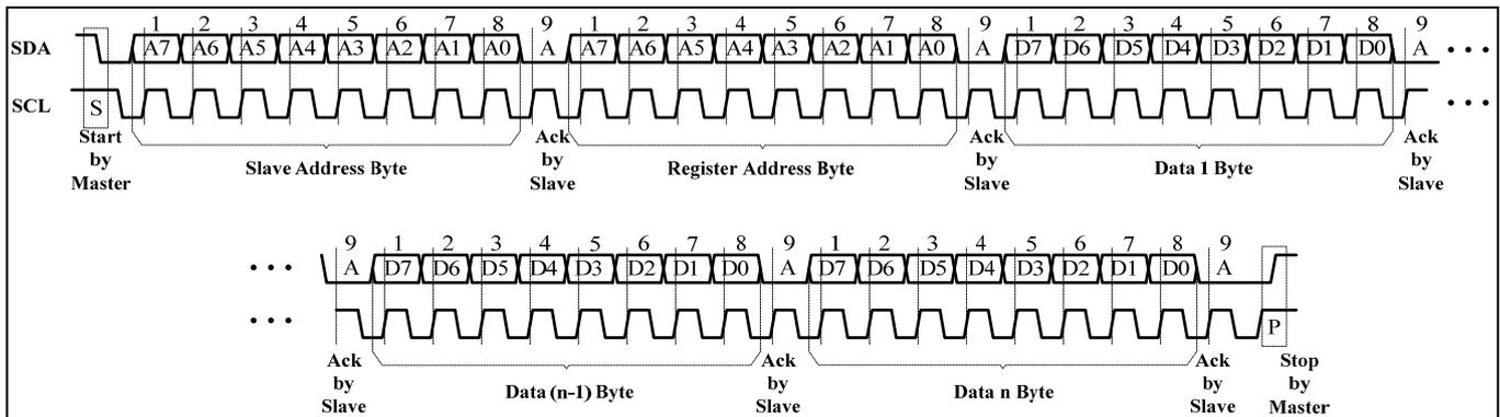
Figure 5 Writing to IS31FL3218 (Automatic Address Increment)
