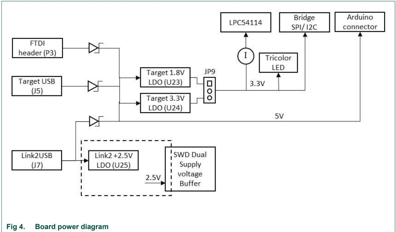
Fig 4. Board power diagram
