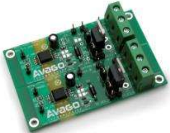
ACPL-H342/K342 Gate Driver with Active Miller Clamp
