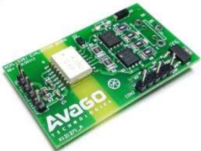
ACPL-339J MOSFET Buffer Interface Gate Driver
